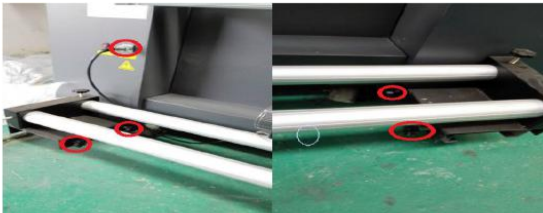
C: Remove the baffle plate
